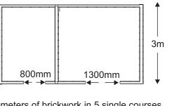
179 meters of brickwork in 5 single courses, tie bonded throughout = 800 bricks (Ibstock ivanhoe burnt)
